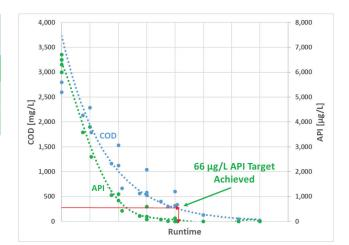
Figure 1 - Treatment reduction curves for API and COD concentrations before, during and after Axine treatment of an antimicrobial API
