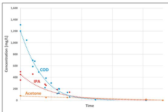
Figure 1 - Baseline wastewater treatment reduction curves for IPA and COD concentrations before, during and after Axine treatment of IPA
