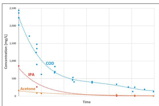
Figure 2 - Spiked wastewater treatment reduction curves for IPA and COD concentrations before, during and after Axine treatment of IPA
